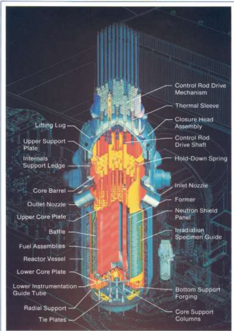
Figure 3.1-1. Cutaway of a Typical Reactor (Four-Loop Plant)
